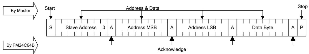
Figure 5. Byte Write
